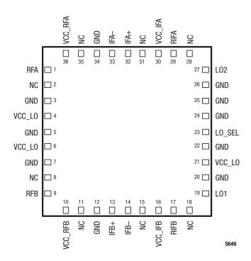
Figure 2. SKY73023 Pinout - 36-Pin MCM
