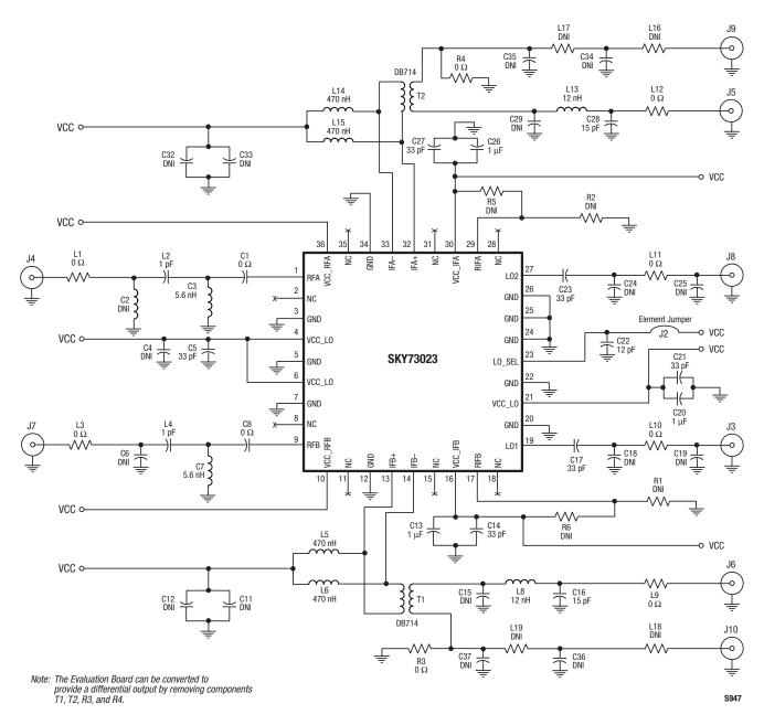
Figure 5. SKY73023 Evaluation Board Schematic
