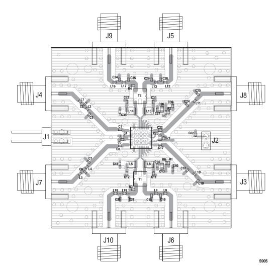
Figure 3. SKY73023 Evaluation Board Assembly Diagram
